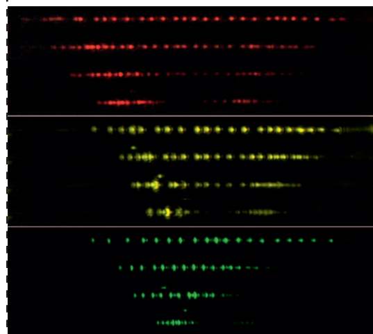
An example of optically self-arranged colloidal waveguide. The distance between the particles is tuneable by the width of two counter-propagating beams which is followed with different spectral properties of the whole structure shown at red, yellow and green wavelengths
