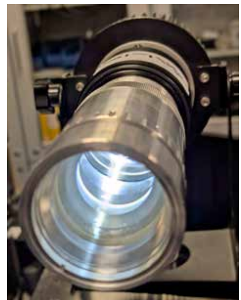
High-resolution projection objective for imaging systems.
