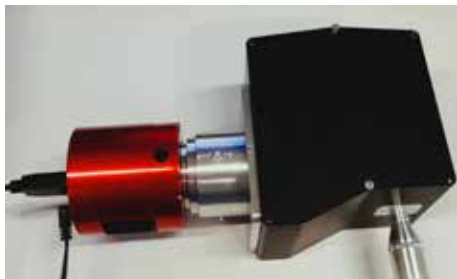
Custom-designed Czerny–Turner spectrometer for Raman spectroscopy of plants.
