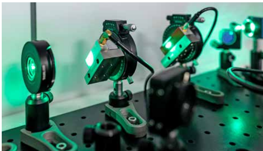
Detail optical path of in-house developed two-photon lithograph.
