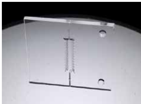
Planar Paul trap with 3D segments manufactured by selective laser etching.
