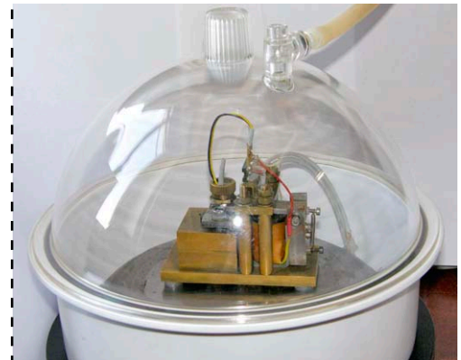
Impact tester in chamber with controlled atmosphere
