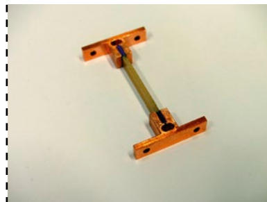
Example of an epoxy composite sample for thermal conductivity measurement in our dedicated apparatus.
